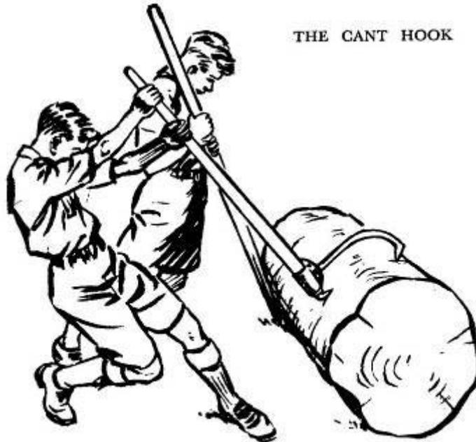
The cant hook is a semi-mechanical lever. The principle is a lever spar and at the working end there is a sharp point known as the 'lip' which digs into the side of the trunk and a curved hook ending in a sharp point set at right angles to the line of the hook which digs into the
