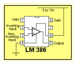
The LM 386 is an 8-pin Audio Power Amplifier Minimum supply voltage 5v Maximum supply voltage 15v
