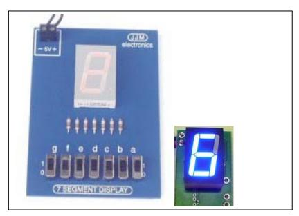
The project above from JJM turns on each segment of the display to show how each letter and number is produced. The second photo is a white 7-segment display.
