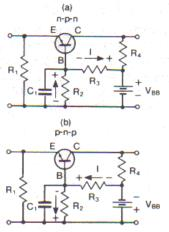
Biasing network for common-base circuit
