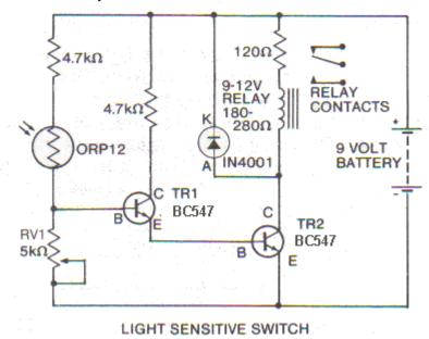
The LDR should be an ORP12 or similar. The relay should have a pull in voltage of 9V or lower and a coil resistance of 280 ohms or higher.
