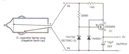
The output will drive transistor radios, cassette players etc. If the current drain is over 500mA, it is a good idea to put a heat sink on  $Q_1$ . Mounting the converter in a metal box with  $Q_1$  on the lid (but insulated from it with a mica washer) will act as a good heatsink.
