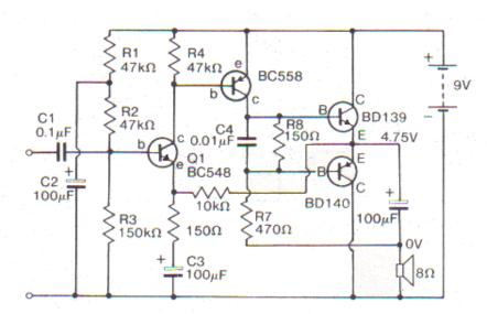
The circuit is for a low power amplifier using a BD139/140 pair in the output stage. The amplifier has a gain of 66. It needs 100mV input for full output, which is approximately 500mW into 8 ohms.
