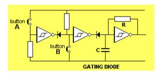
The second diode is called the **gating diode**. When the output of the second inverter is LOW, the capacitor is prevented from charging as the diode will not allow it to charge higher than 0.7v, and thus the oscillator does not operate. When the output of the second inverter is HIGH, the capacitor is allowed to charge and discharge and thus oscillator will produce an output. If the push buttons can be placed together, the circuit can be simplified to:
