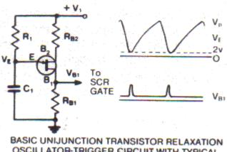
OSCILLATOR-TRIGGER CIRCUIT WITH TYPICAL WAVEFORMS
