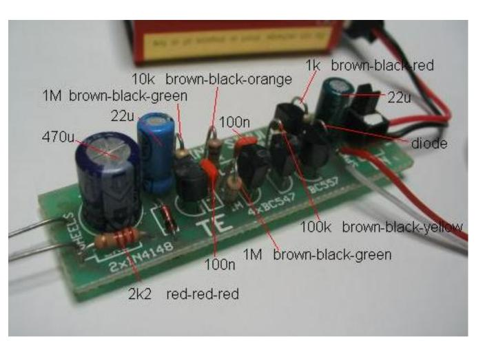
A realistic steam sound can be generated with a 4-transistor directly-coupled amplifier connected to a small speaker. The "white noise" is generated by the breakdown across the junction of a transistor and it is activated by a switch made up of contacts touching the wheel of one of the carriages. As the train speeds up and slows down, the sound corresponds to the movement. See Talking Electronics website for the full project.
