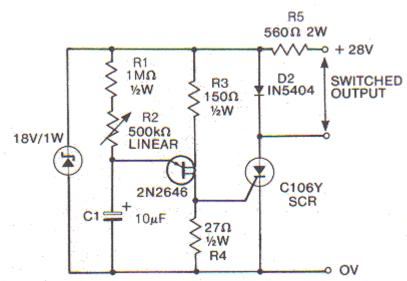
Initially the SCR is off. The timing sequence is started by shorting out C1. C1 then charges through R1 and R2 until the UJT triggers, developing a pulse across R4 which turns on the SCR. Holding current for the SCR is supplied by current through R5 and D2. When the SCR triggers, it pulls the voltage across the UJT to <2 volts. This discharges C1.
