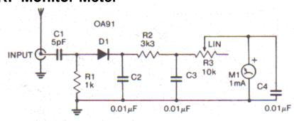
The circuit is an RF monitor meter suitable for measuring the strength of a signal from transmitters. You could use it to measure the effectiveness of different antennas for example. It works in much the same way as the crystal set, but without the tuned circuit. The meter M, will indicate the strength of the 'carrier'. Modulation of the carrier i.e. signal on the carrier, will cause the reading to vary. M, is not critical, and any meter of 1mA or better sensitivity will be suitable.
