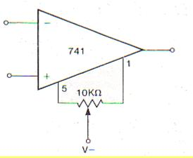
This can be important in DC circuits or where a high impedance feedback resistor is used. A 10k ohm variable resistor is connected between pins 1 and 5 (of the 8 pin package) and the wiper is taken to - supply.
