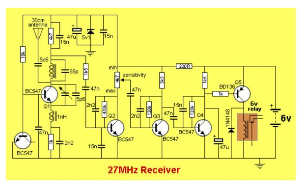
This is a single channel receiver, similar to the circuit above. It can be modified to turn on a "latch" a relay. This means the relay can be turned on remotely but it cannot be turned off. The second circuit shows the modification to turn the relay ON with a short tone and OFF with a long tone.
