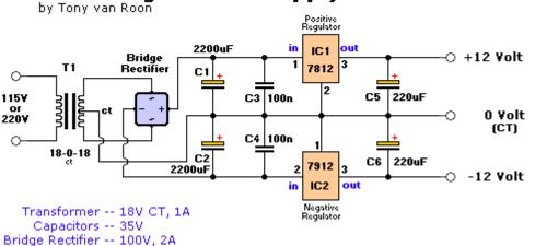
The use of a pair of the regulators (positive and negative) makes an ideal dual rail supply, for powering op-amps etc. A suitable circuit is shown below. This one uses 12V regulators, but obviously the voltage can be varied by changing regulators.
