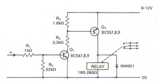
The circuit will work with any relay with a coil resistance higher than 180 ohms and a pull in voltage of less than 12v.
