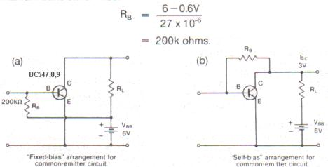
This arrangement is sensitive to temperature and varying gains of transistors. A better arrangement is shown above (b). This stabilizes the operating point of the transistor because an increase in collector current drops the collector voltage and thus decreases the base bias.
