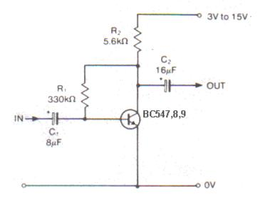
This circuit will operate on any supply from 3v to 15v. Using a 9v supply, the circuit gives a voltage gain of 46dB (200 times), frequency response within 3dB from 30Hz to 100kHz, input impedance of 1.5k ohms and an output impedance of 5.6k ohms. The base bias resistor  $R_{\rm 1}$  gives sufficient negative feedback to compensate for the large variation of  $h_{\rm FE}$  values in individual transistors and for variations in supply voltage.
