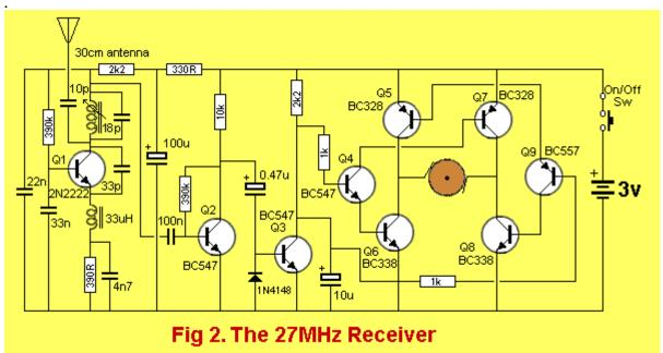
Here is the circuit from a 27MHz remote control car. It is a simple single-channel link that activates the car in the forward direction when no carrier is being received, and the motor reverses when a carrier is detected. See Talking Electronics website for more details - 27MHz Links.
