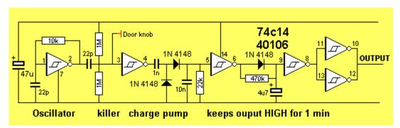
The output of the above circuit can be taken to an alarm. Open the reed switch contacts and connect the reed switch to the output of the Door-knob alarm.
