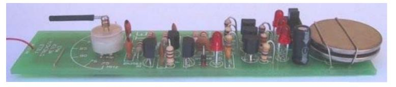
A field strength meter is a very handy piece of test equipment to determine the output of a transmitter. Talking Electronics website describes a number of Test Equipment projects to help with developing your projects.
