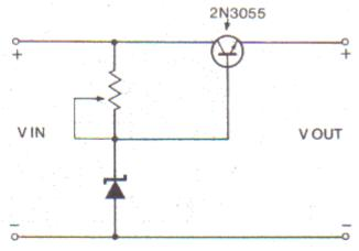
The output voltage of this circuit will be equal to the zener voltage minus the base-emitter voltage of the transistor (approx. 0.7V).
