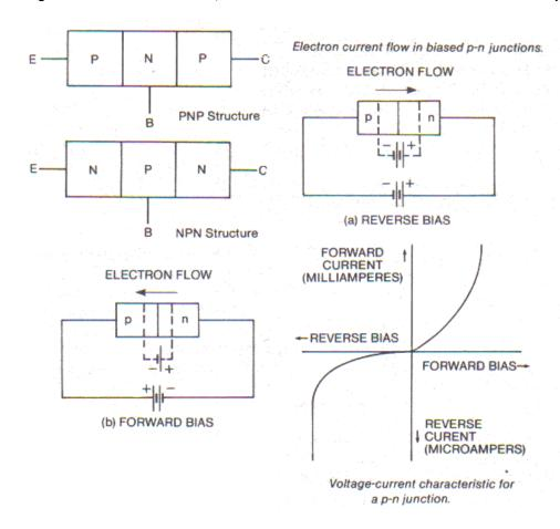
If another layer is added to the semiconductor junction, the resulting device becomes a bipolar transistor. The three layers of the device are the emitter, the collector and the base. In normal operation, the emitter to base junction is forward biased and the collector to base junction in the reverse direction.
