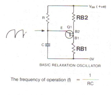
The design of the UJT trigger is very broad. RB<sub>1</sub> is limited to values below 100 ohms for most applications. R<sub>1</sub> should be a value between 3k and 3M. Supply voltage can be from 10 to 35v. If the circuit is being used to trigger an SCR, RB<sub>1</sub> must be low enough to prevent DC voltage at the gate from exceeding the maximum voltage that will not trigger the SCR. In practice, keep R<sub>B</sub>, below 50 ohms.
