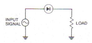
Simple diode rectifying circuit.
