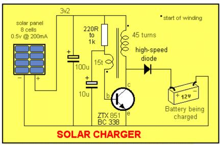
This solar charger can be used to charge a 12v battery from any number of solar cells. The circuit automatically adjusts for any input voltage and any output voltage. See Talking Electronics website for the full project.
