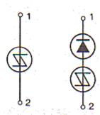
SYMBOL OF ASYMMETRICAL AC TRIGGER SWITCH (ST4) AND EQUIVALENT CIRCUIT
