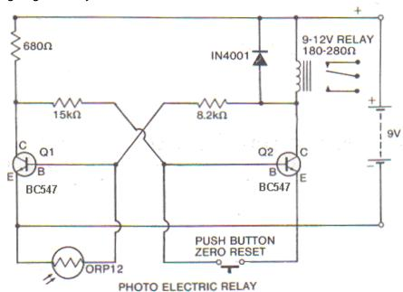
The relay should have a coil resistance of 180 ohms or higher and a pull in voltage of 9V or lower
