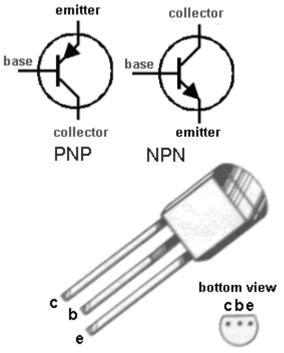
Low frequency, general purpose small signal transistors widely used in audio, switching and television circuits. The BC547-9 series and BC557-9 series are functionally identical to the common BC107-9 series.
