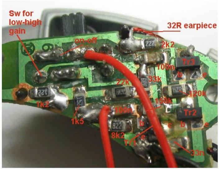
The surface-mount 3-Transistor amplifier
